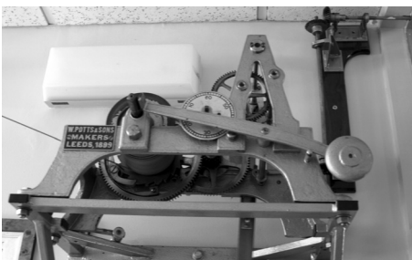
Originally manufactured by Potts of Leeds in 1899, the clock was an amalgamation of parts. The movement from Ilkley station was restored by Graham Oliver and mounted at the top of the stairs outside the lounge door and connected to the faces by a long rod across the full width of the building.
